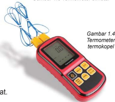
Gambar 1.4 Termometer termokopel
