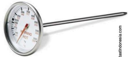
Gambar 3. Termometer bimetal
